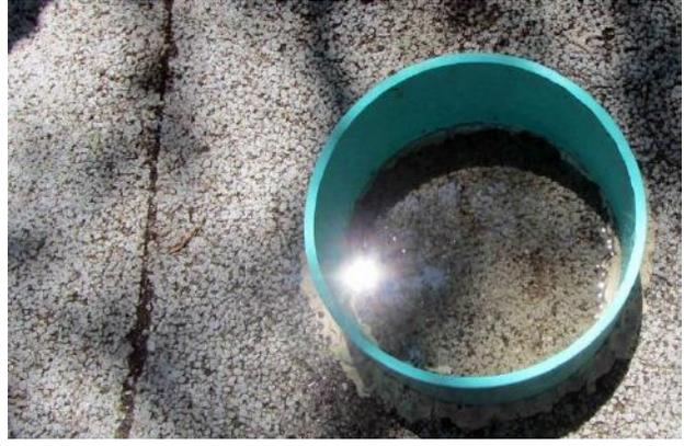
**Figure 5. Initial or pre-wetting test using ASTM C1701 on pre-cast pervious concrete panel in the street parking lane. Note the standing water due to a clogged surface.**
