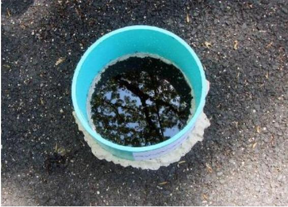
**Figure 4. Initial or pre-wetting test using ASTM C1701 on porous asphalt alley. Note the standing water due to a clogged surface.**
